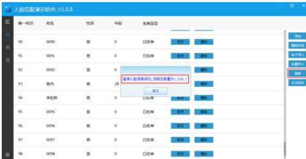
8.6. Manually synchronize the face database: Click the [Manual Sync] button to manually synchronize the face database in the face recognition device and the demo software face database to avoid the face matching software face database and device face after replacing the device. The library is inconsistent, causing the identification comparison information to be displayed incorrectly. After replacing the new device, you must first manually sync the face database.
